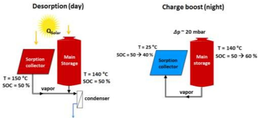
Figure 2: Working principle of the sorption collector under typical boundary conditions
