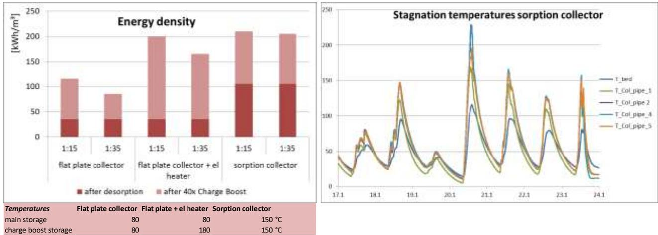
110 Figure 4: Left: Improvement of the energy density based on repeating the charge boost mode compared to the conventional desorption at the same temperature under different mass ratios between charge boost storage/sorption collector and main storage and different use cases (temperatures). Right: Measured stagnation temperature of the prototype sorption collector
