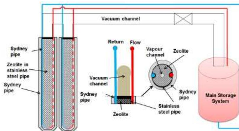
Figure 1: Concept of sorption collector applied as charge boost storage
