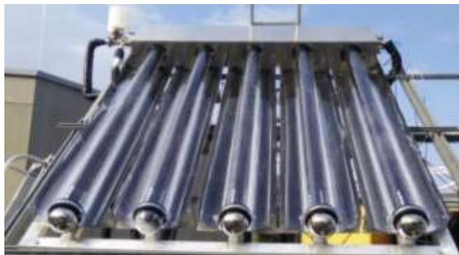
Figure 3: Developed prototype of sorption collector with glass tubes
